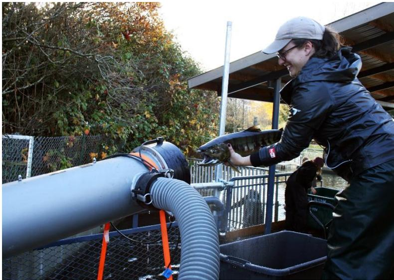
Fish ladders require on average 5-10% of a dam's water to operate and are an exhausting journey for fish. Fish transported via Whooshh's system (a suspended, pliable, water-filled tube) spend mere seconds being gently transported compared to hours and possibly days of arduous climbing up a fish ladder. This leads to higher egg viability when spawning upstream and lower mortality rates as compared to fish
