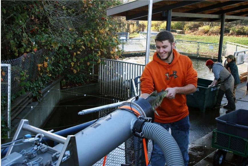
In addition to its uses in hatcheries, Whooshh technologies also help fish navigate more easily over obstacles such as dams. Fish ladders can be an exhausting journey for fish. Fish transported via a Whooshh system spend mere seconds being gently transported, compared to hours and possibly days of arduous swimming to climb up a fish ladder. Reducing stress and conserving the energy of the fish
